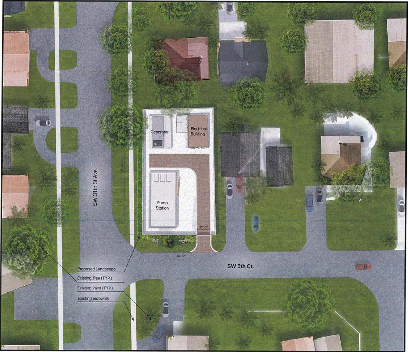
Figure 10: : Proposed Stormwater Pump Station – Option 3 (City Property)
