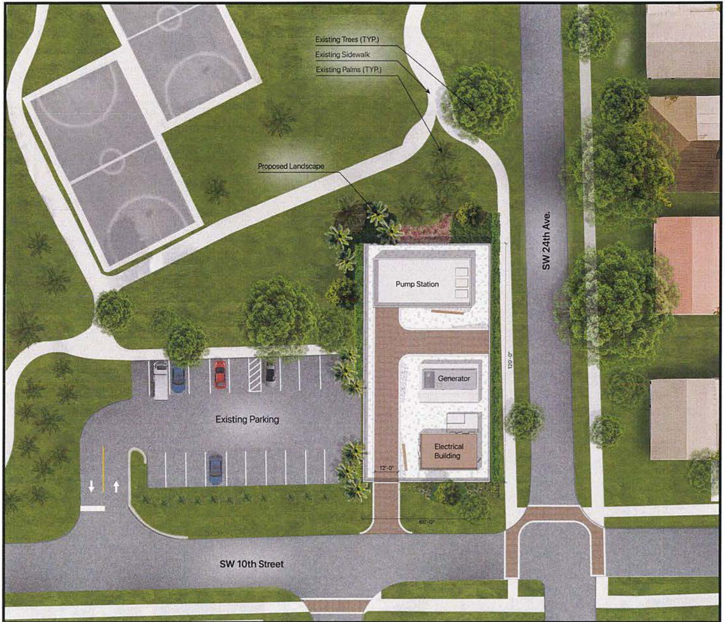
Figure 8: : Proposed Stormwater Pump Station (Riverland Park)
