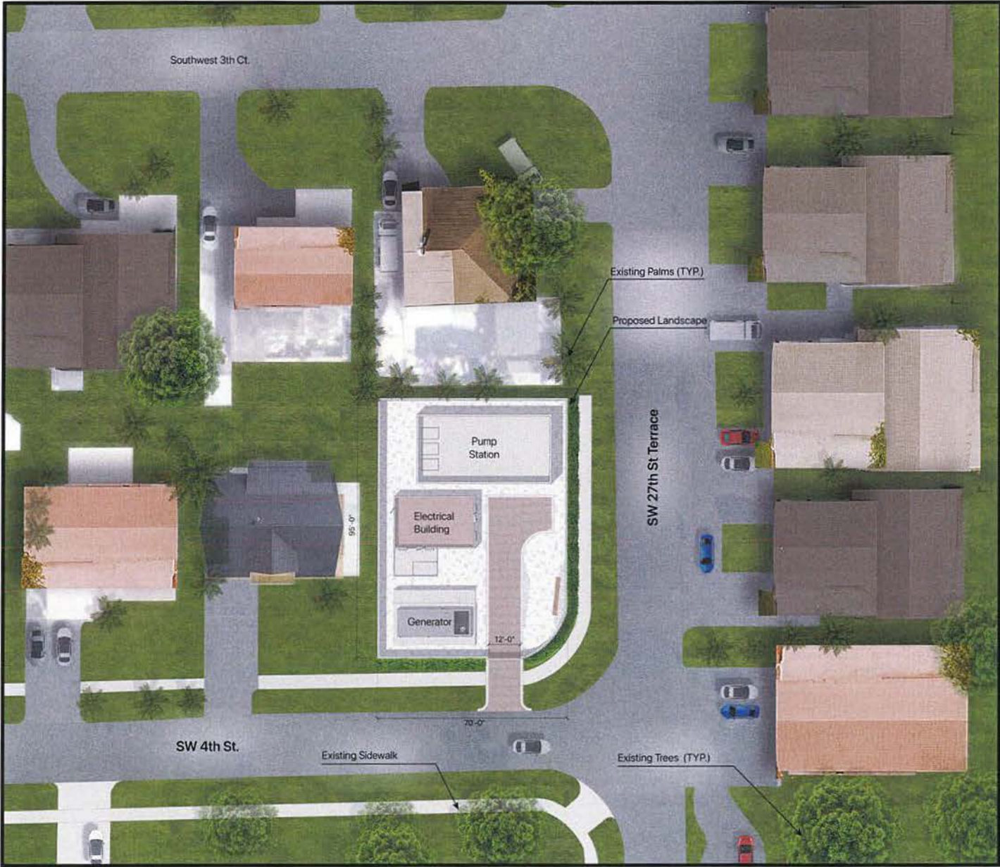
Figure 9: : Proposed Stormwater Pump Station – Option 2
