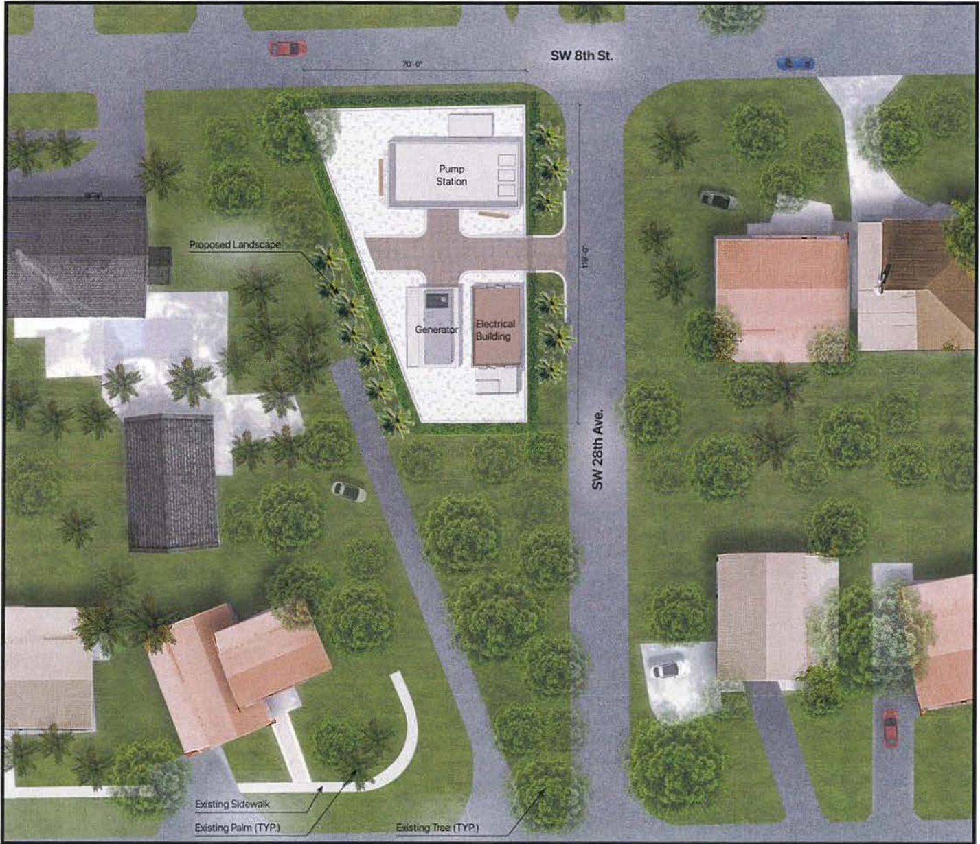
Figure 8: : Proposed Stormwater Pump Station – Option 1
