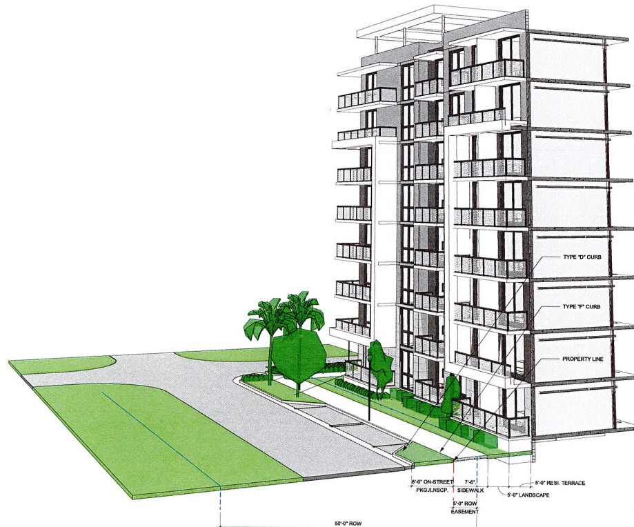
1 PROPOSED STREET SECTION - SECONDARY STREETS (NW 7TH STREET SHOWN) N.T.S.
