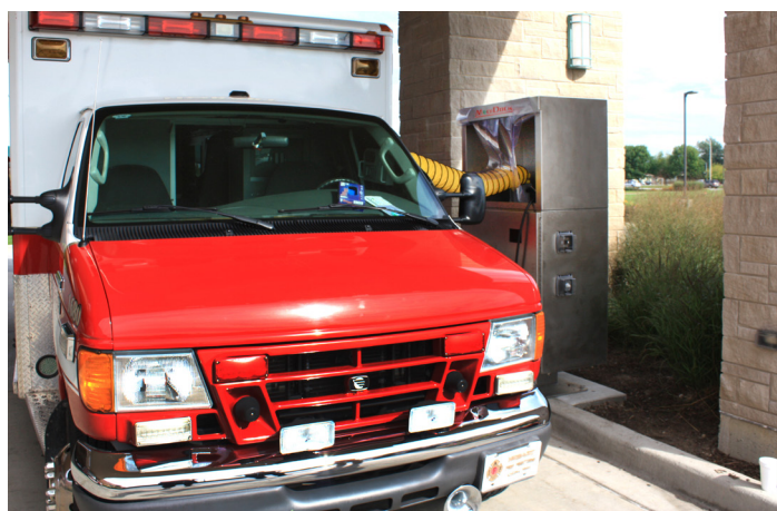
Ambulance hooked up to a MediDock, which provides power and conditioned air. Used with permission of American Idle Reduction, LLC.
