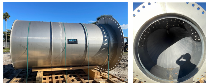
A newly installed 72" tidal valve in the Historic Dorsey Riverbend neighborhood. This valve discharges into the New River and helps reduce flooding during high tide events.
