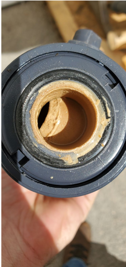
Source: Photos of lime carryover provided by the City of Fort Lauderdale
