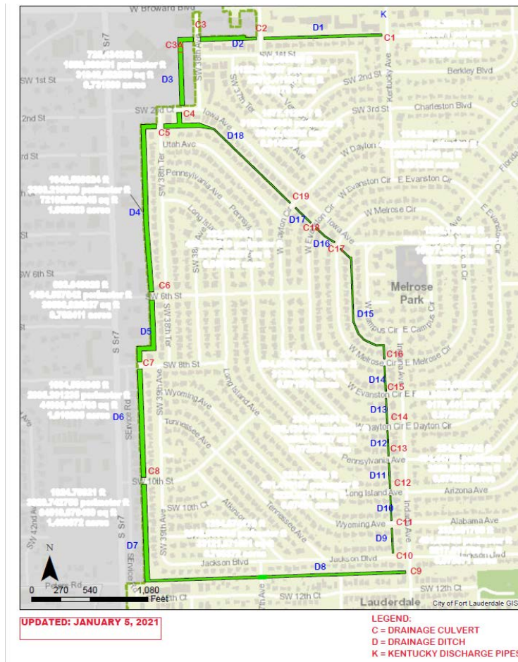
Figure 3: Culverts and Drainage Ditch Segments in the Melrose Park Neighborhood
