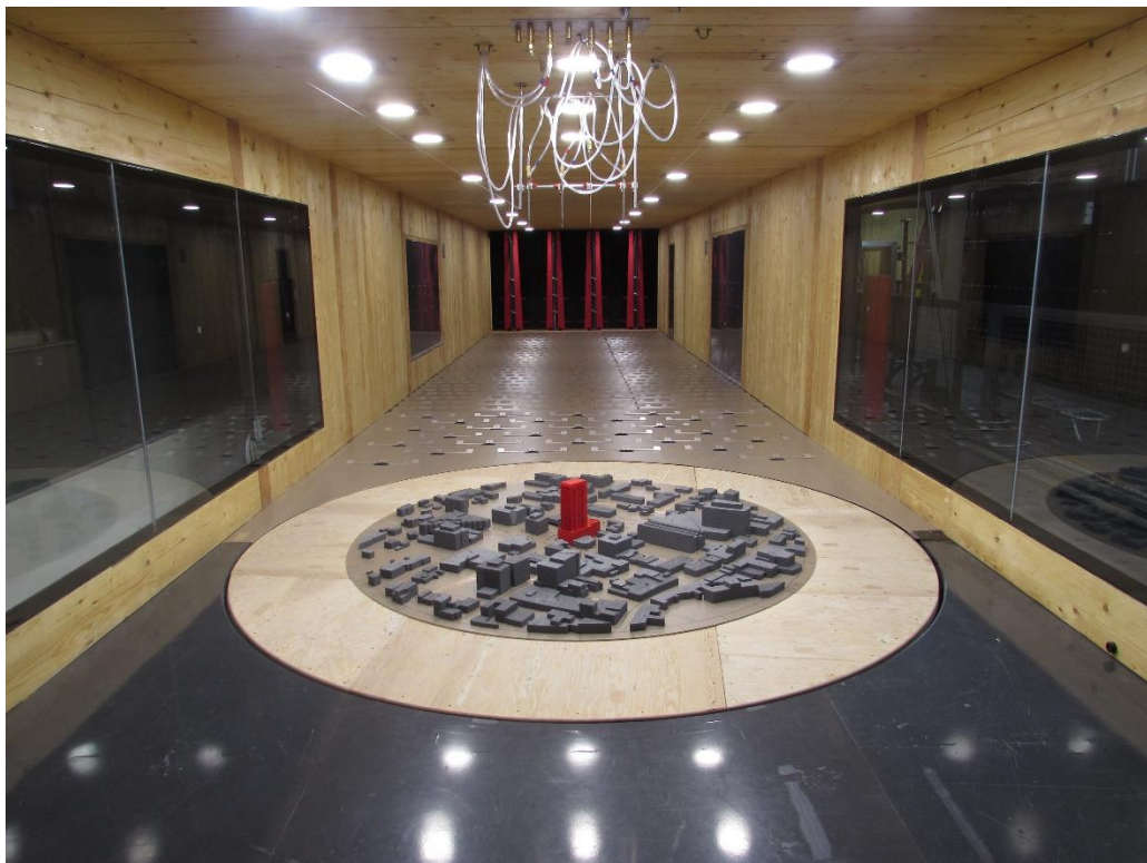
Image 3: Example Study Model in a Boundary-Layer Wind Tunnel
