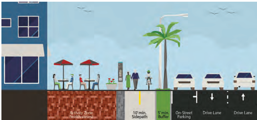
Side Path Typical Section: Urban Core
