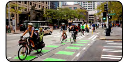
Cycle Track Dashed Intersection Markings Style
