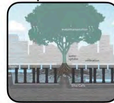
Resiliency - Silva Cells for Stormwater Management
